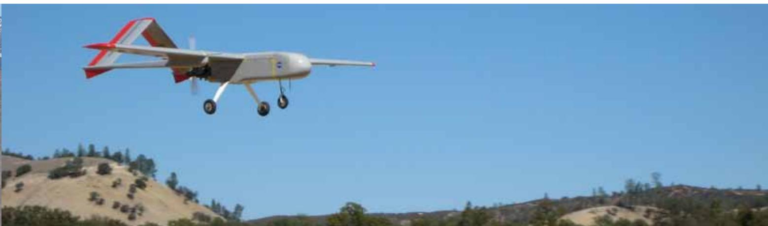
The SIERRA sent position, temperature, and humidity data to the ground. Through real-time processing, the information was displayed within the Google Earth™ Mapping Service, allowing researchers to revise course plans and protect the aircraft from icing conditions during flight. The combination of satellite data and real-time data from the SIERRA allowed many researchers to contribute to the mission without traveling to the region.
