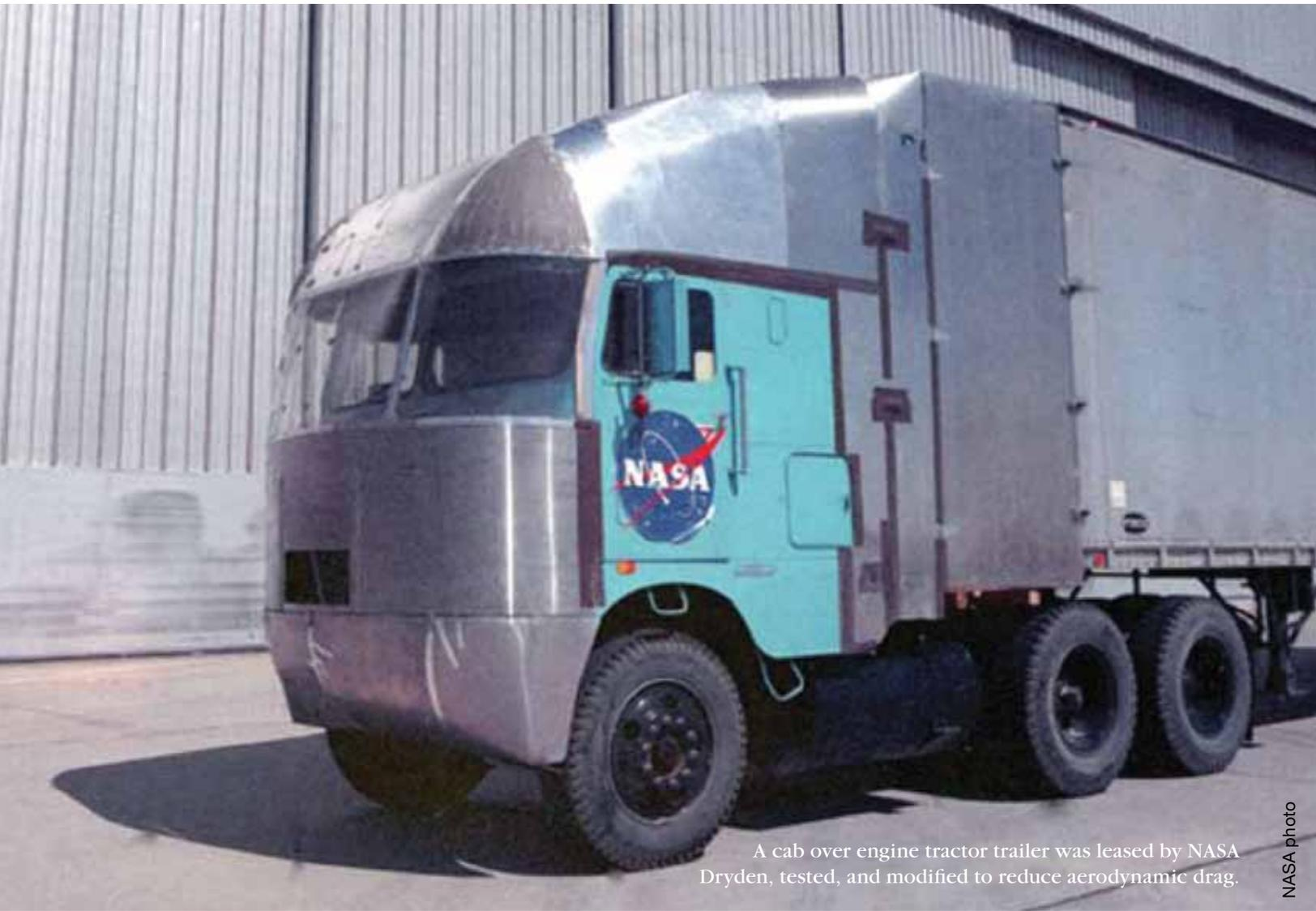
A cab over engine tractor trailer was leased by NASA Dryden, tested, and modified to reduce aerodynamic drag.
