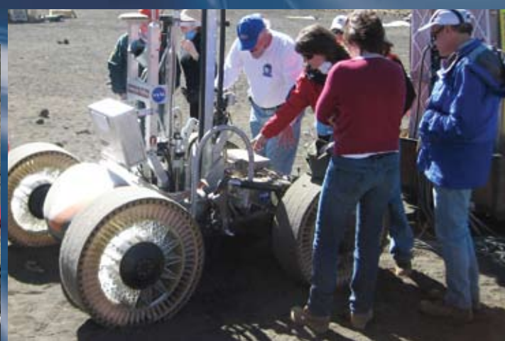
Prototype robotic lunar resources prospector
