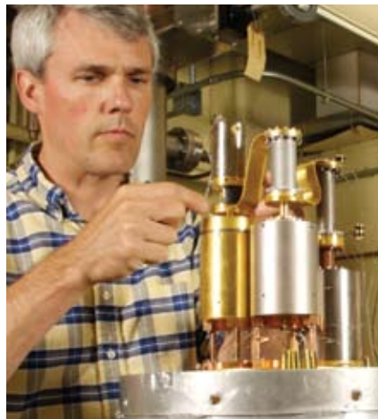
GSFC researcher Peter Shirron works on his continuous adiabatic demagnetization refrigerator (ADR)
