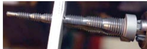
*Drilling a test piece of previously damaged leading edge material with a prototype step-tap drill bit*
