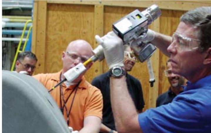
*Crew training using the step-tap drill bit in the Pistol Grip Tool (PGT) drill driver on a Shuttle leading edge test article*
