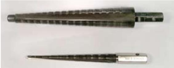
*Flight-certified, step-tap drill bits for threaded holes that stop at the required size step*
