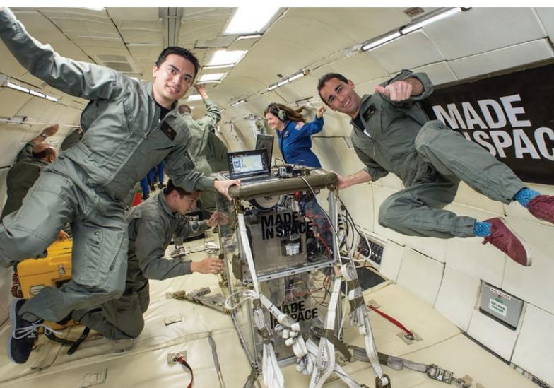
The Made In Space 3-D Printer was validated during parabolic flight testing.
